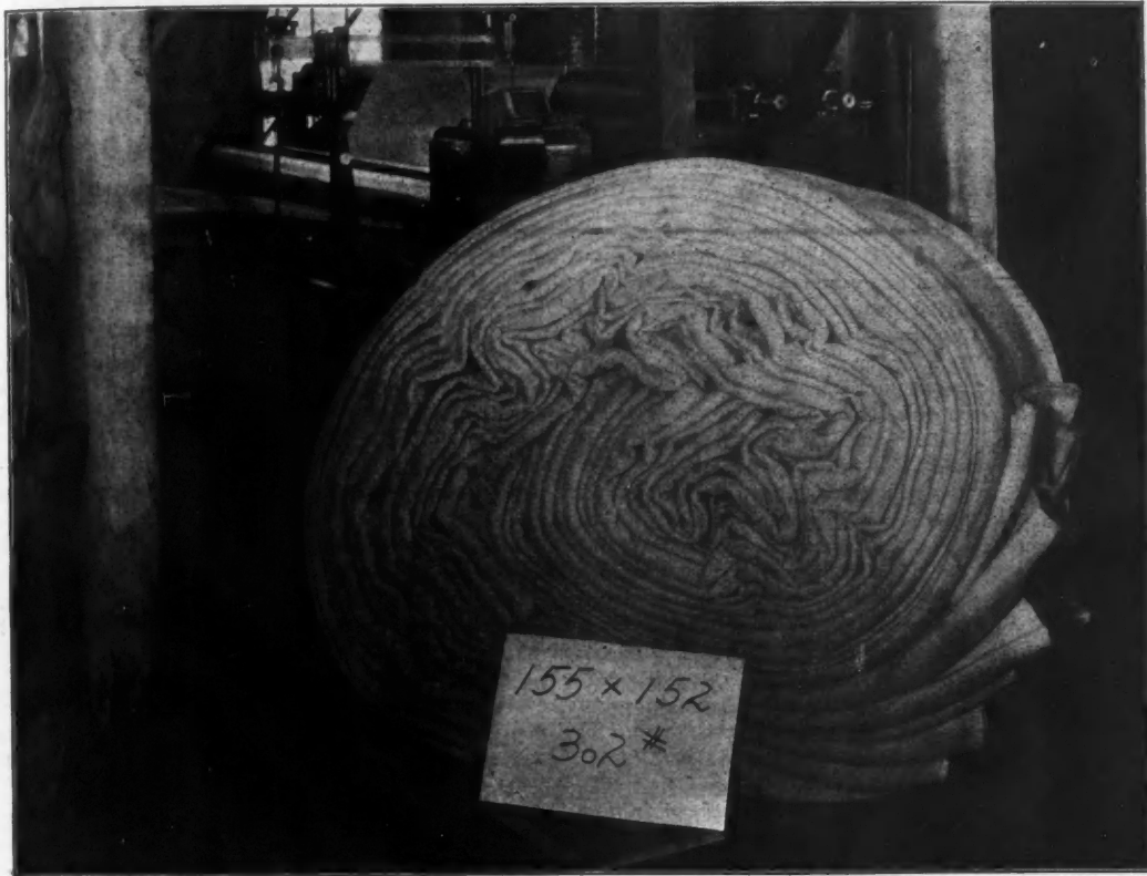
A 155x152" finished cylinder wet felt on the scale.
