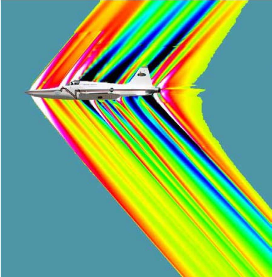
A color-coded illustration of high-pressure shock waves and lower pressure expansions based on imagery that was generated by the Computational Fluid Dynamics (CFD) program used by its SSBD team in designing the F-5's modifications. A photo of the modified aircraft in flight has been inserted to complete the illustration. (Illustration: NGC, Photo: NASA)
