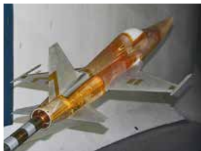
Ten percent model of SSBD in Northrop Grumman's low-speed wind tunnel, October 2002. (NGC)
