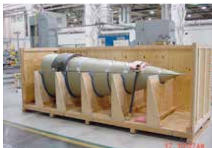
Nose bulkheads and framework being assembled and later crated for shipment with skin panels attached. (NGC)
