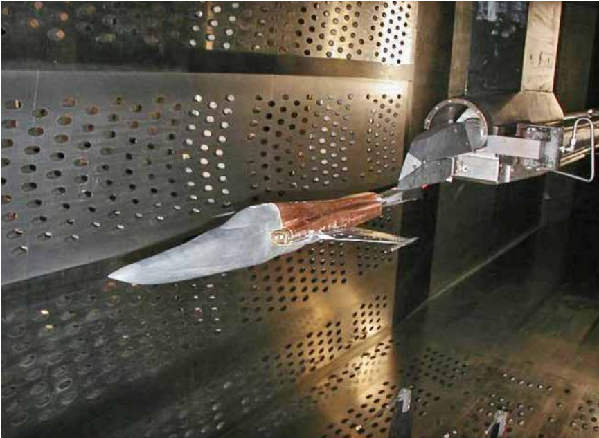
Improved SSBD wind tunnel model and mounting mechanism, May 2002. (NGC)
