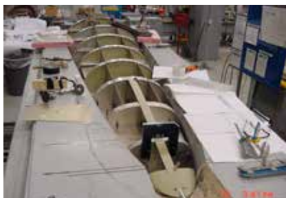
Nose bulkheads and framework being assembled and later crated for shipment with skin panels attached. (NGC)
