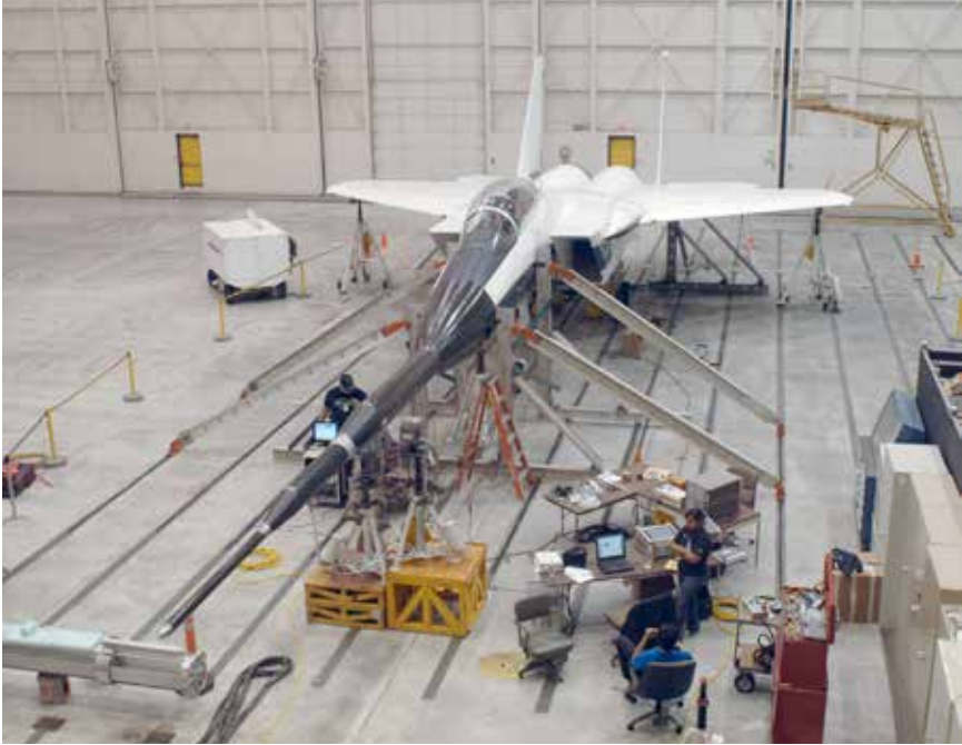
F-15B no. 836 during vibration testing of Gulfstream's Quiet Spike at the Dryden Flight Research Center. (NASA)
