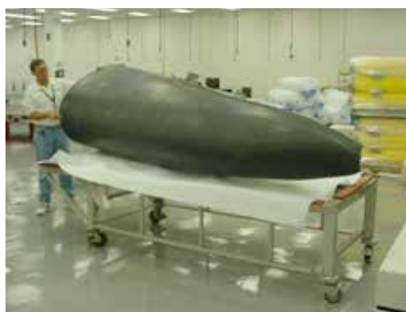
Preparing tooling (top) to form the outer mold line of the nose glove (bottom) in August 2002. (NGC)
