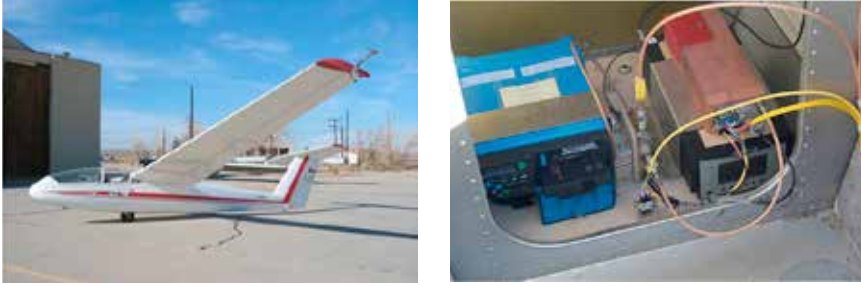
Blaik L-23 sailplane with microphone on left wingtip and installed recording equipment. (NASA)
