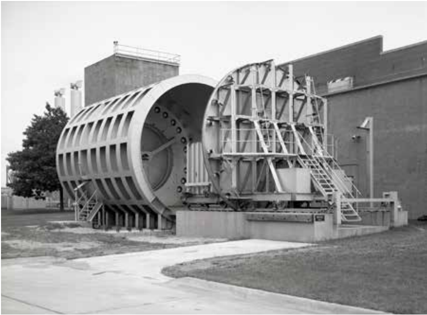
Langley's Low-Frequency Noise Facility, built originally for testing the extremely loud sounds of Apollo booster rockets. (NASA)
