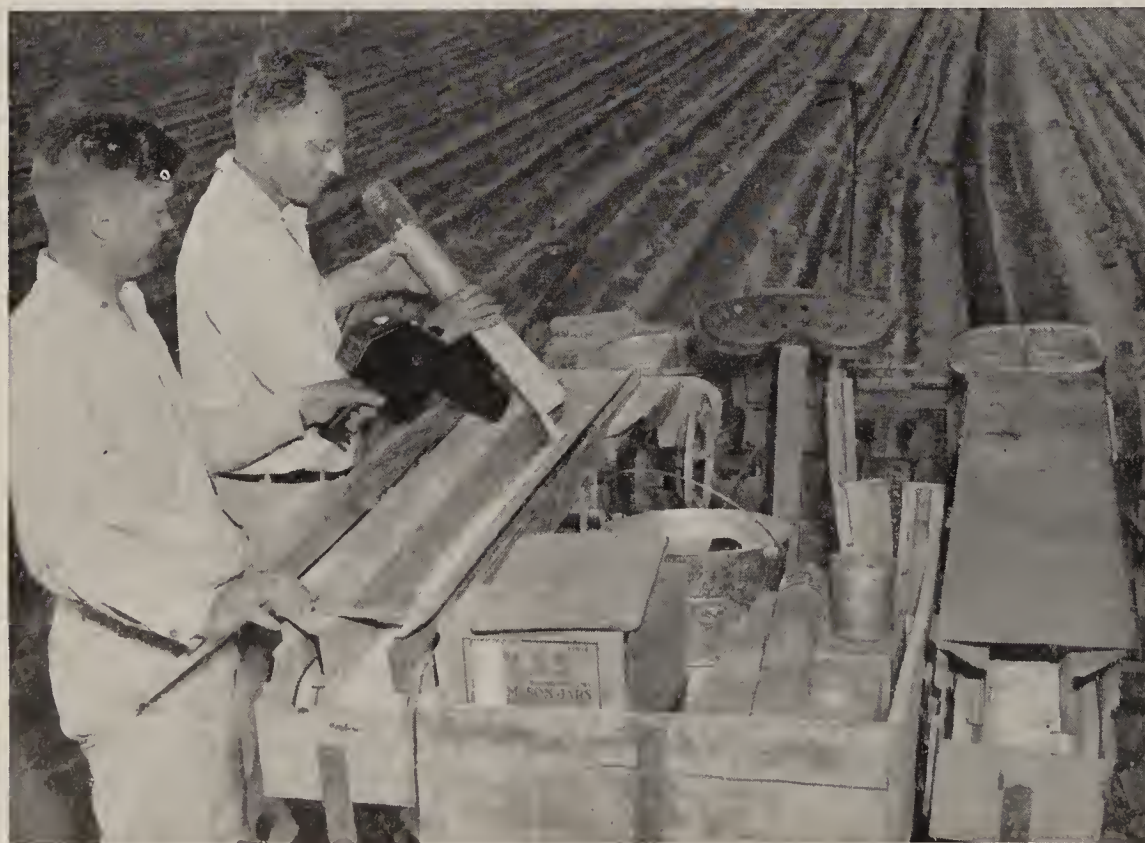
Radioactive fertilizer to be utilized by corn plants is checked with safety meter for radiation. This work goes on at the Research Division of the U. S. Department of Agriculture at Beltsville, Md.
