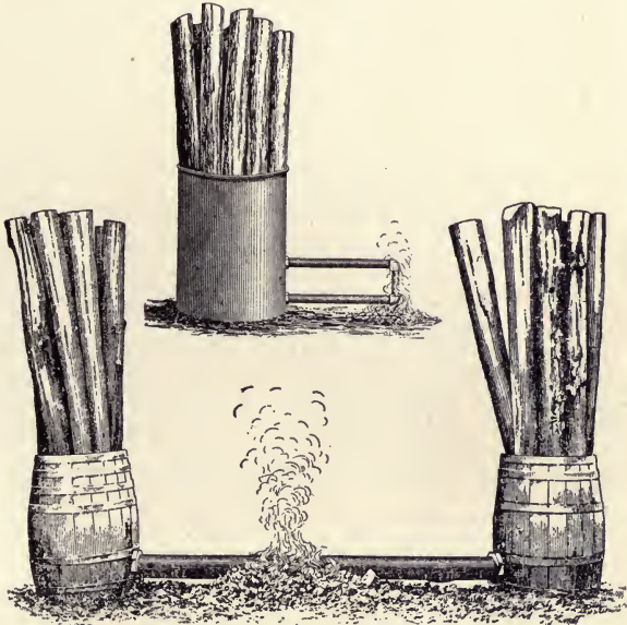
FIG. 77.—Simple apparatus for treating posts. 1
