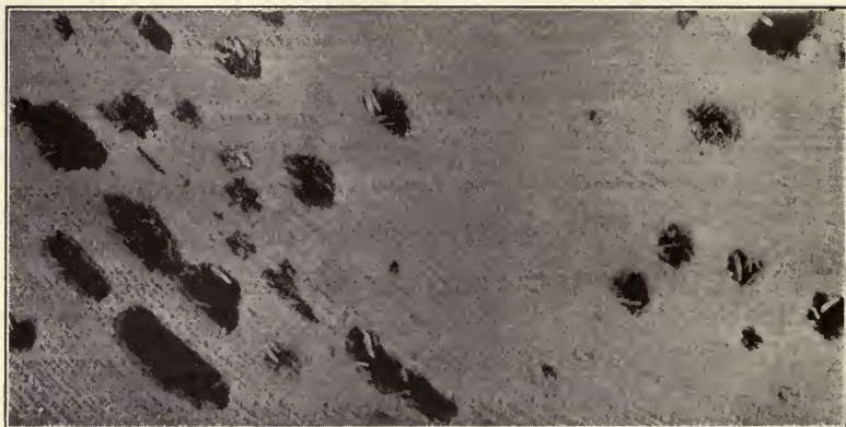
FIG. 44.—Section of wood cut from cypress after attack by wood-destroying fungus ( Dedalea vorax ).
