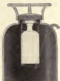
FIG. 46.—Section through portable fire extinguisher.
