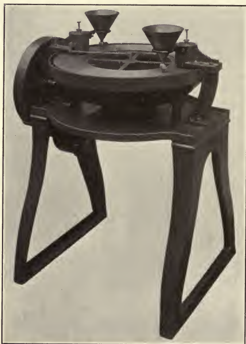
FIG. 39.—Dorry machine for making abrasion tests.
