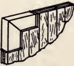
(a) Application of Tin to Corners of Fire Door.
