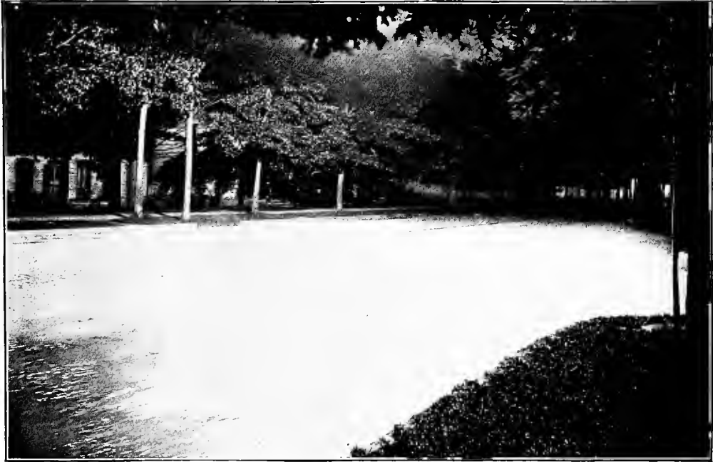
Figure 21—Distribution of light from an A. C. 6.6 ampere enclosed lamp.
