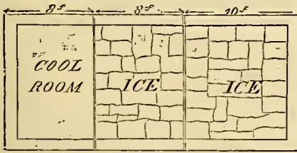
Fig. 3.—PLAN OF UPPER PART OF ICE-HOUSE.
