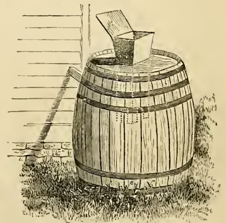
Fig. 1.—CASK FOR HOUSE SEWAGE.
