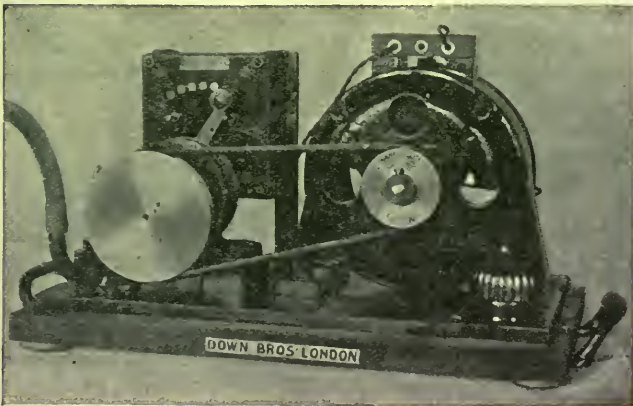
FIG. 47.—Motor actuating Mr. Kelly's insufflator.
