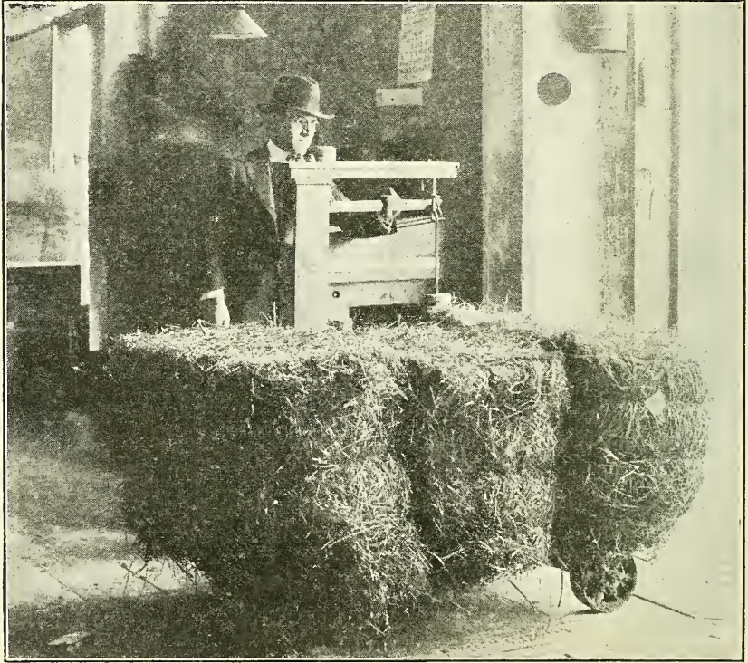
FIG. 3.—Weighing on dormant warehouse scales. Trucks are usually used when weighing on such scales, and care should be taken to see that tare weights of all trucks used are uniform and that proper tare is allowed.
