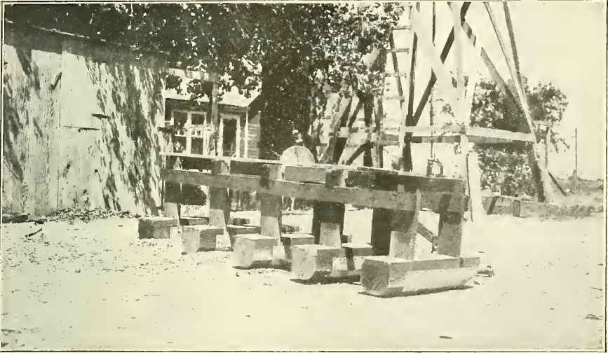
FIG. 1.—A SLEDDING IMPLEMENT USED IN SMOOTHING IRRIGATING FURROWS IN SUGAR-BEET FIELDS, BEING SOMETIMES HELPFUL IN DISTRIBUTING THE WATER.
