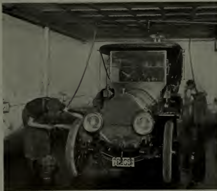
Wash your car with a gently flowing stream of cool water. A forceful stream knocks off the mud and carries along pieces of varnish too
