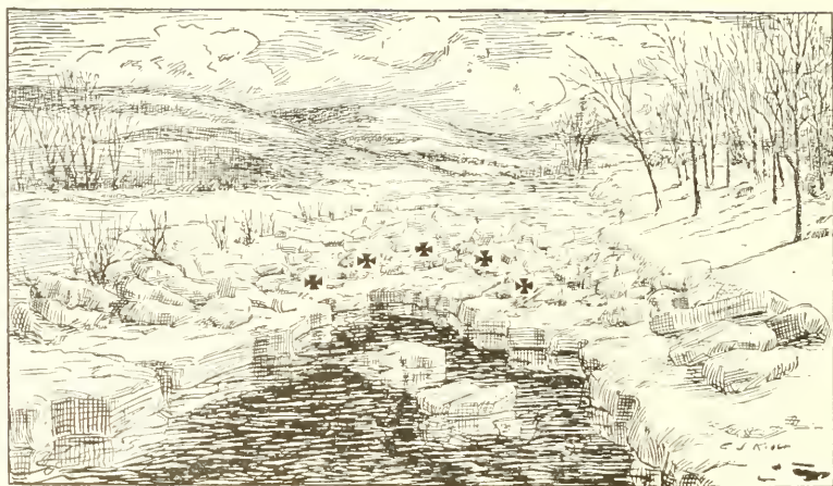
DIAGRAM SHOWING LOCATION OF ROW OF HOLES FOR BLASTING AN ICE GORGE
