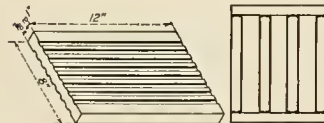
Fig. 928—1 inch Slabs for End Construction. Showing form in which Slabs are usually made. A tap on the corner separates the tile into slabs.
