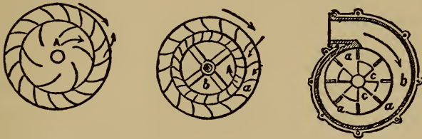
Figs. 191, 192, 193. Central discharge and turbine wheels
