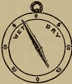
Fig. 71. Index of Hygrometer
