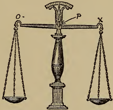
Fig. 6. Double lever as scales
