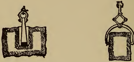
Figs. 205, 206. Lewis bolts, for lifting stones
