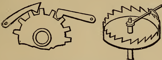
Figs. 144, 145. Intermittent circular motion
