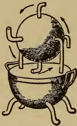
Fig. 30. Hero's steam engine
