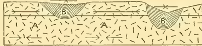
FIG. 1.—Diagram of assumed conditions of compressive strain in rocks in a basin of accumulation. AA, massive crystalline rocks. BB, the rocks of the basins. The arrows indicate the direction of the compressive strains; the spaces between their heads indicate the measure of the yielding at the several points.
