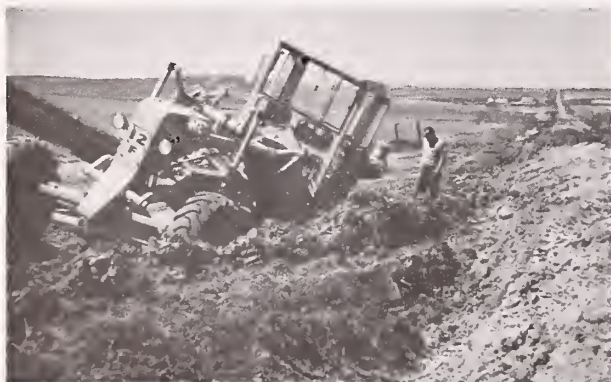
FIGURE 2.—Nothing warned the operator that a potential saline seep existed beneath the surface.
