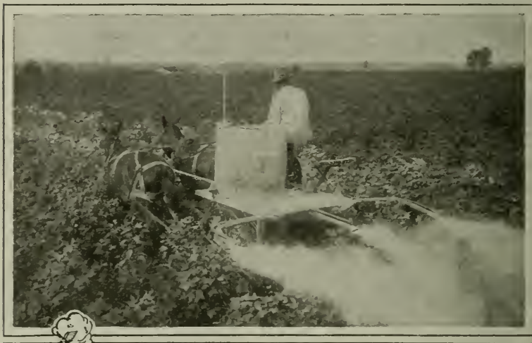
Cart Duster in Operation in Cotton Field.
