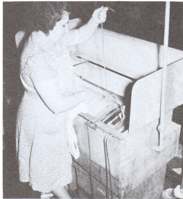
PH 3046. Poor practice in dipping a rack and metal parts into the cleansing solvent, the fumes of which are toxic.
