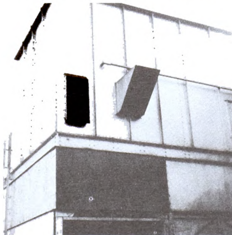
PH 3204-D. The above special enclosed sand-blasting chamber is not only equipped to protect the worker inside, but to prevent dangerous silica dusts from clouding the surrounding atmosphere.
