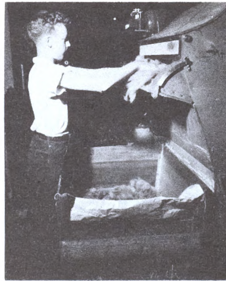
PH 2940-C. In the new automatic type of forming machine, one hat is weighed automatically by means of an electric eye.
