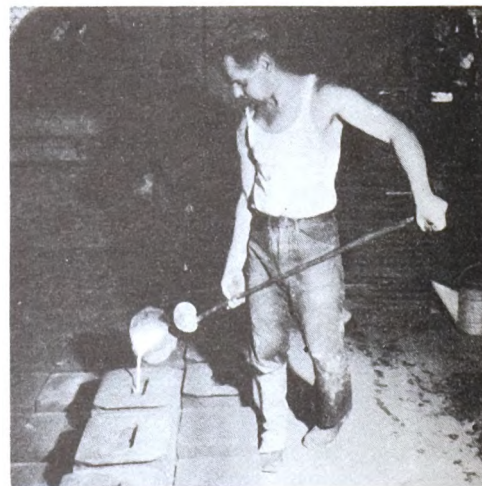
PH 3059-E. The safety leggings of chrome leather, reinforced with steel can be removed with one swift jerk in case the molten metal splashes the pourer's leg.
