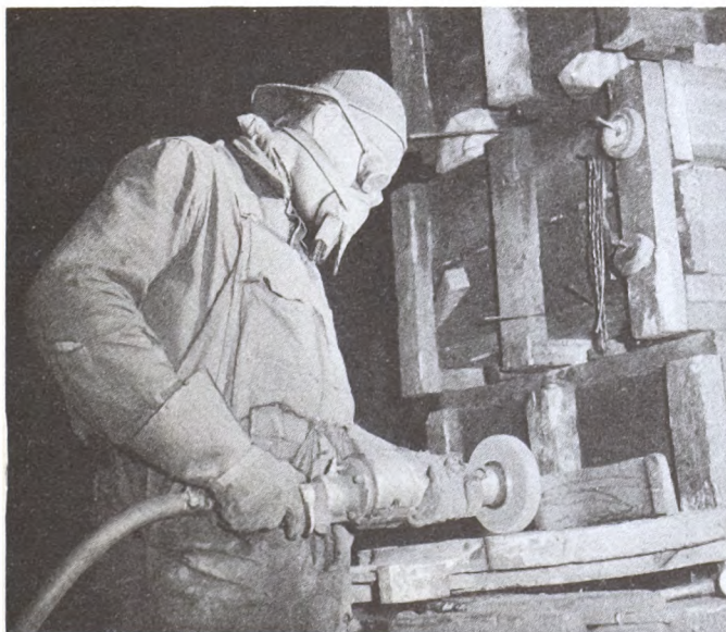
PH 3197-D. Some jobs in a foundry cannot be protected by special ventilation equipment. In operating a portable electric grinder the approved type of mask and goggles give adequate protection.
