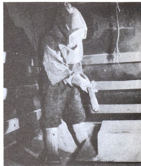
PH 3201-D. Not a man from Mars, but an American war worker wearing a modern approved air-line respirator, gloves, leggings, and special steel-reinforced shoes.
