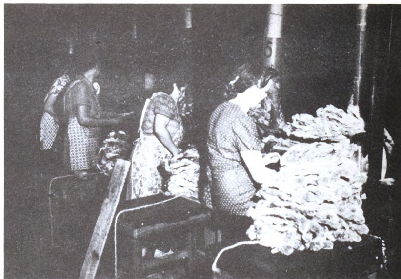
PH 3005. Shaving the rabbit hair from the skins which have been dried in the open air. Exhaust ventilation is needed to control dust from carrotted rabbit fur.
