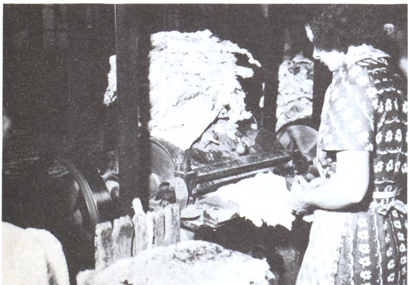
PH 2989-C. Close-up of the shaving operation. Note piles of skins on top of machine, an indication of crowding and poor housekeeping.
