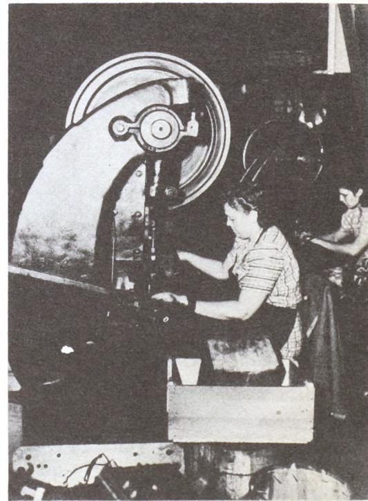
PH 3012. Machines too close together, unguarded machinery, and poor housekeeping make dangerous working conditions.
