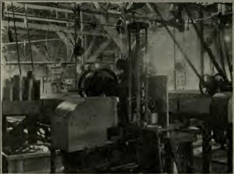
Guarded knuckle mechanism on can closing machine.
