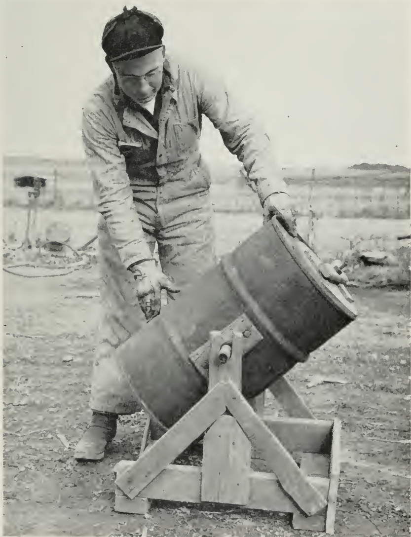
Fig. 55.—Oil drum seed treater. This is one type of device that can be used to treat seed with dust, slurry, or liquid fungicides. (Photograph from Emil Mosser, Farm Adviser, White County.)
