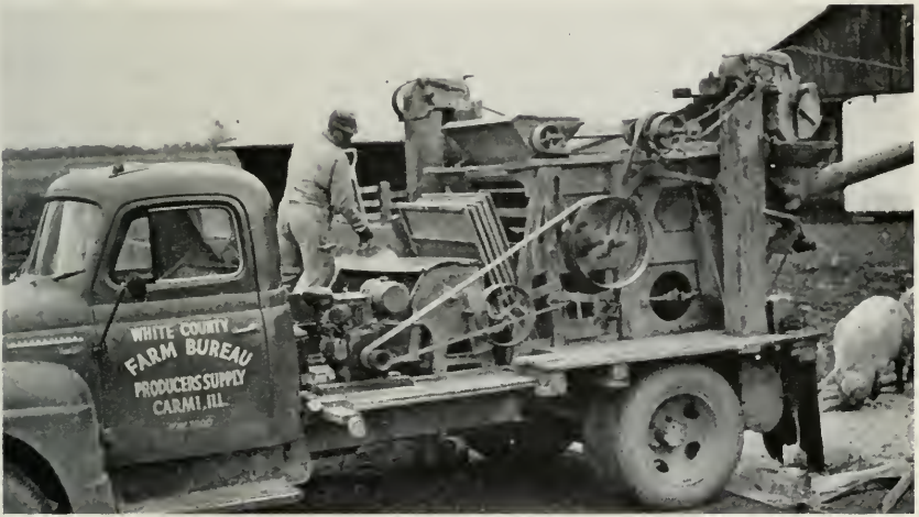
Fig. 56.—Seed cleaner and treater mounted on a truck. It treats about 55,000 bushels of seed a year. (Photograph from Emil Mosser, Farm Adviser, White County.)
