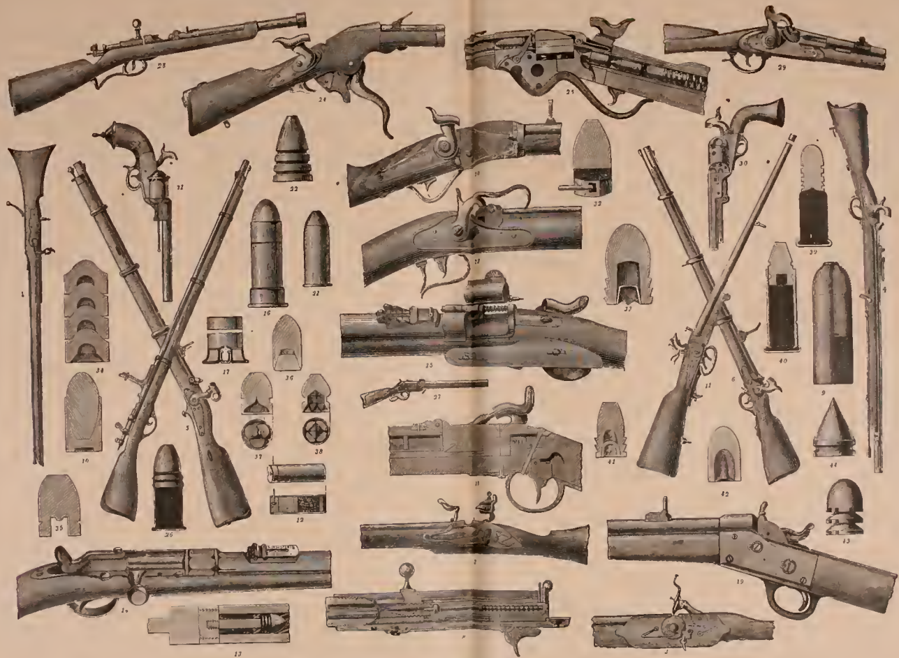
Guns. 1. Gun with match-lock. 2. Rotary-lock. 3. Flint-lock. 4. French hunter's gun. 5. Cossack gun. 6. Italian infantry gun. 7. Prussian needle-gun. 8. Section of lock of Prussian needle-gun. 9. Prussian needle-gun cartridge. 10. Rotary lock. 11. Lefauchaux gun, with shot cartridge. 12. Section of lock of Prussian needle-gun. 13. Boregun gun. 14. Chassepot rifle. 15. English Enfield rifle. 16. Its cartridge. 17. Section of latter. 18. Austrian gun, Wänzel's pattern. 19. Remington rifle. 20. Peabody gun. 21. Cartridge, and 22, ball thereof. 23. Pfeffer gun. 24. Spencer's repeating carbine. 25. Section thereof, and 26, cartridge. 27. Henry's repeating. 28. Prussian needle carbine. 29. American carbine. 30. Colt's revolver. 31. Lefauchaux revolver. 32. Lefauchaux cartridge. 33. Russian Nimis-gun. 34. Bavarian case-cartridge. 35. Bavarian expanding ball. 36. English expanding ball, with wooden plug. 37. French expanding ball, ancient form. 38. Recent form of the same. 39. Swiss ordnance cartridge, with compressed powder. 40. Box cartridge, with peripheral fire. 41. Baden expanding projectile. 42. Ploennis' expanding projectile. 43. Lorenz's compressed projectile. 44. Old pointed projectile.
