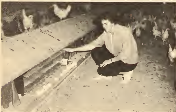
FIGURE 35.—Community nests showing eggs rolled to a belt egg conveyor.
