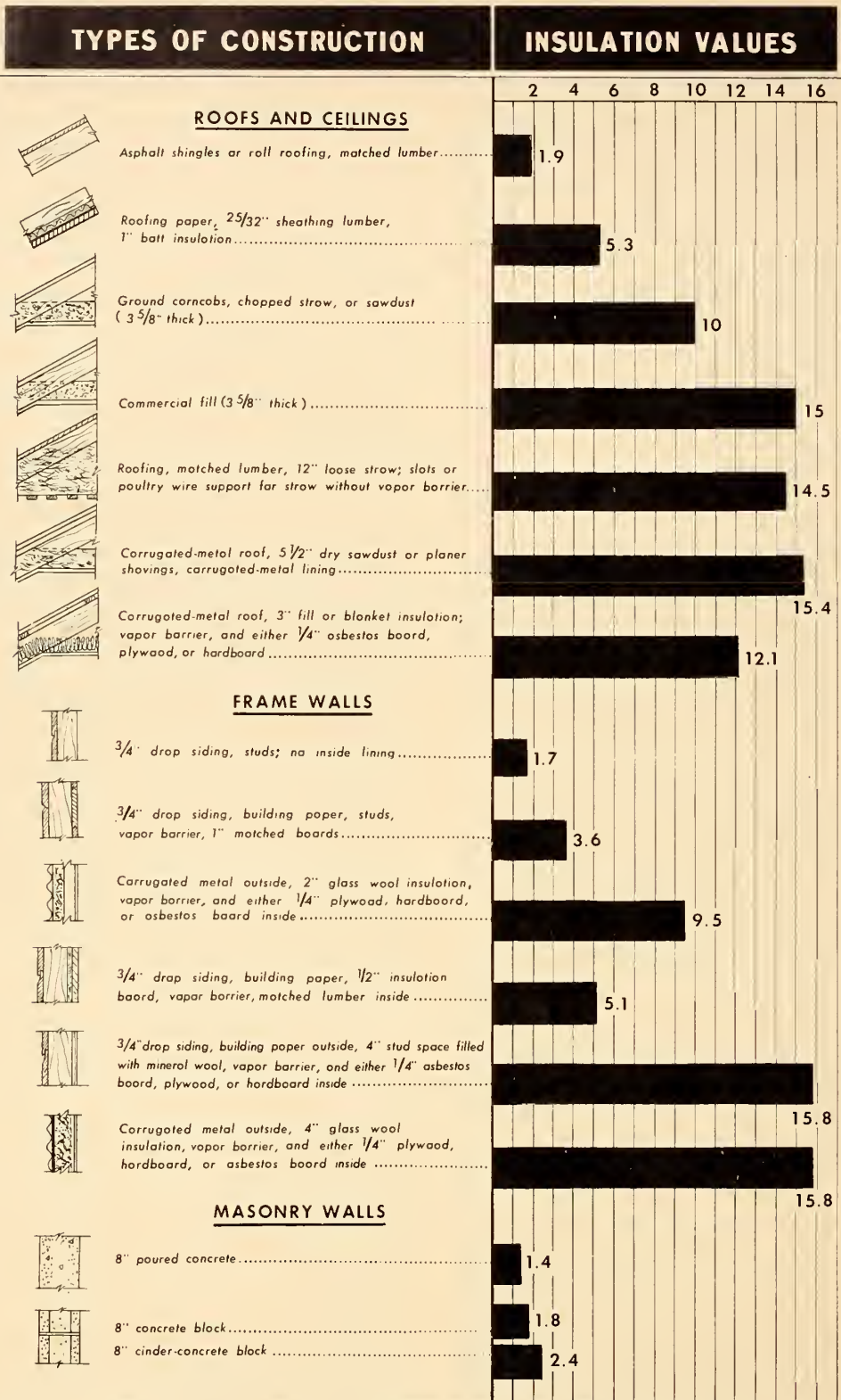
FIGURE 23.—Insulation values for common types of roof, ceiling, and wall construction. All attic spaces are considered ventilated.
