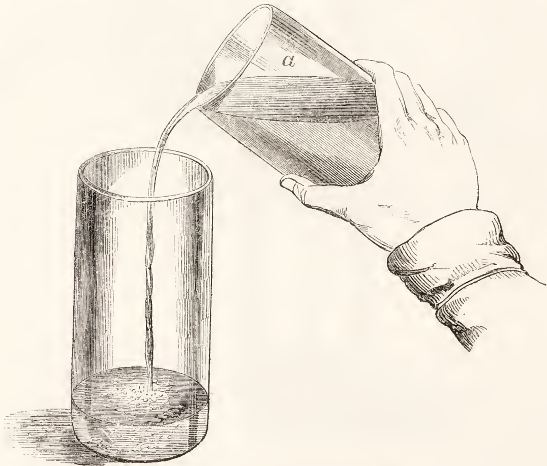
DECANTATION OVER A GREASED RIM.
