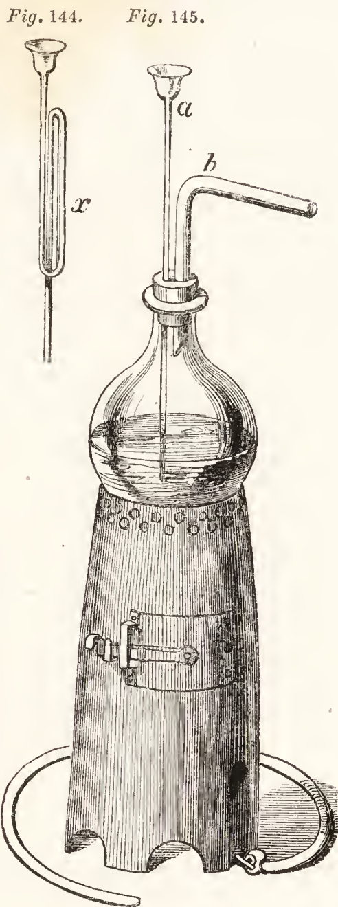
GAS-FURNACE AND FLASK FOR DISTILLATION.
