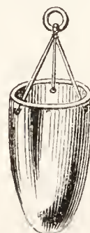
SPECIFIC GRAVITY BUCKET.
