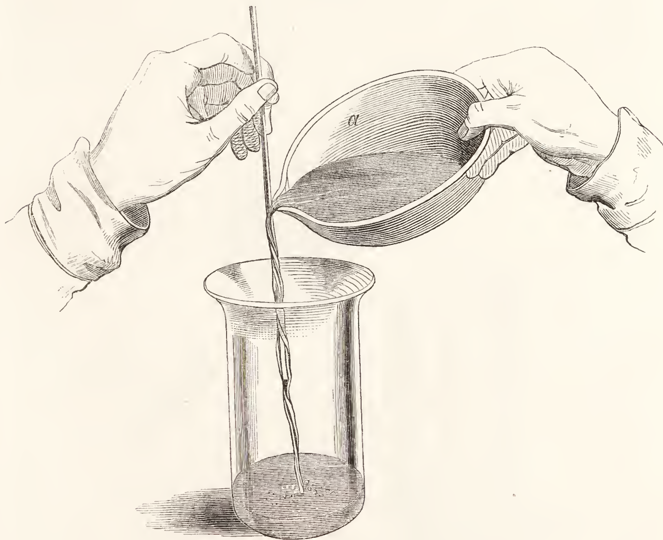
DECANTATION WITH A GUIDING-ROD.
