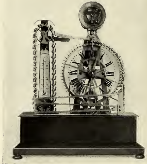
THE CLOCK RUN BY STEEL BALLS.
