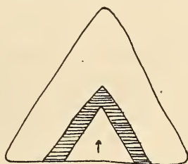
FIG. 11.—Shaded area shows the material removed in solution, to permit the movement of the inner cone.
