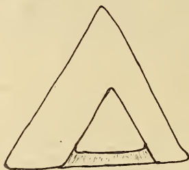
FIG. 10—Shows small cone penetrating large cone which does not show any evidence of displacement in the large cone.
