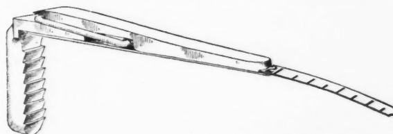
THE HOOK WITH TAPE IN POSITION
