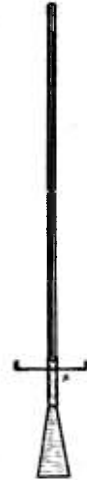
FIGURE 15.—The spud, an effective tool for cutting off weeds with thick roots below the surface of the soil.
