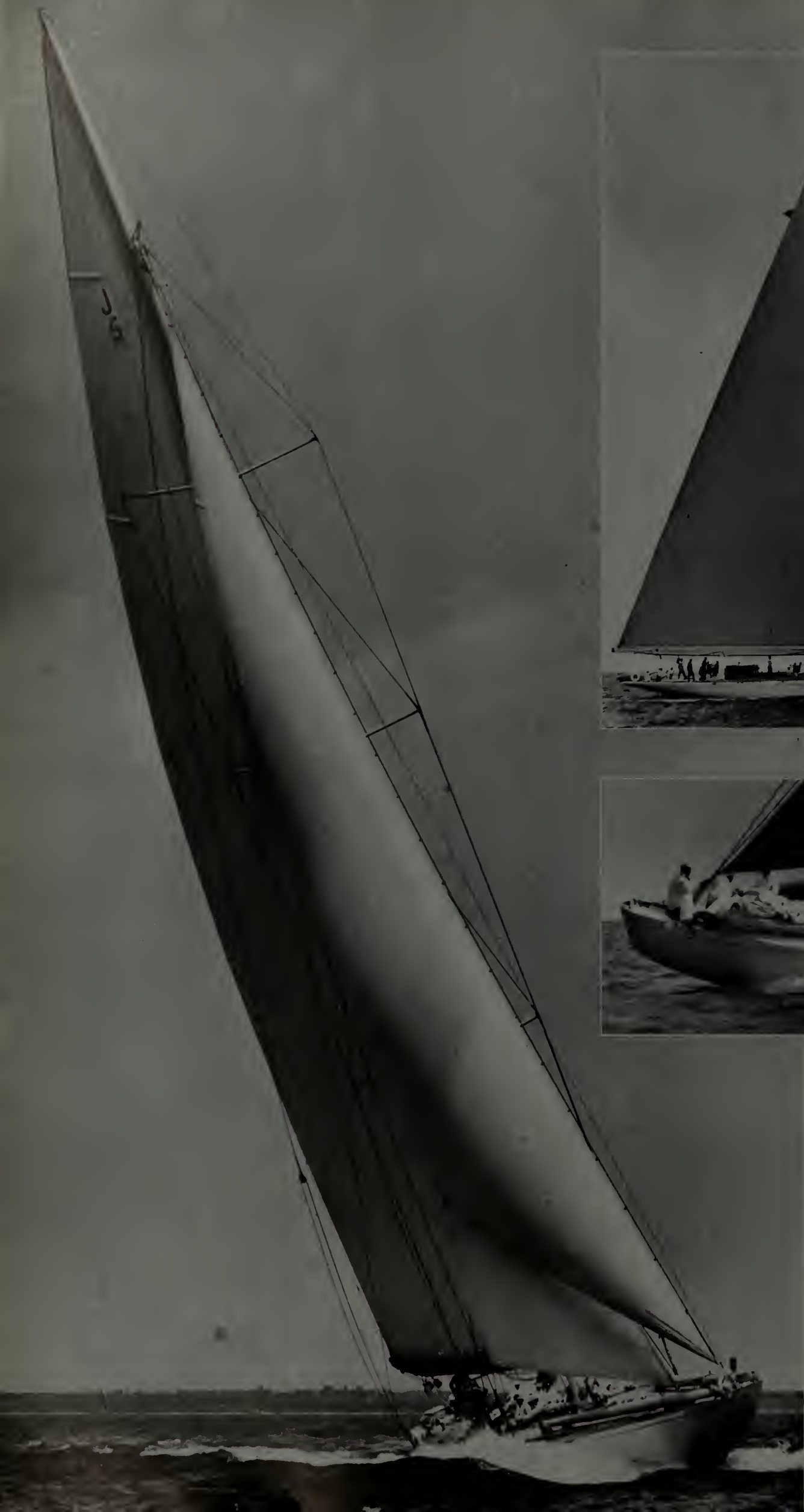
Harold Vanderbilt's "Ranger," outstanding boat in the early trials, shows her lofty rig as she goes to windward. Her snub-nosed barrel bow, while not a thing of beauty, saves weight and gives working deck room forward
