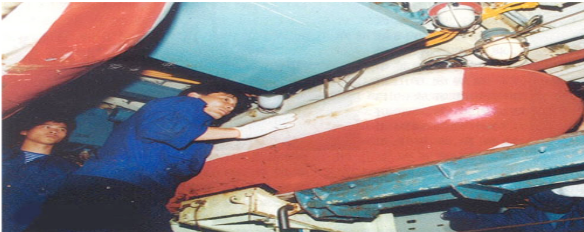
Figure 3. The PLA-Navy's EM52 (T-1) is a submarine laid fast-rising rocket-propelled bottom mine. It is laid in the sea bottom and will rise to the surface using its rocket propulsion and without guidance. (From SinoDefence.com)
