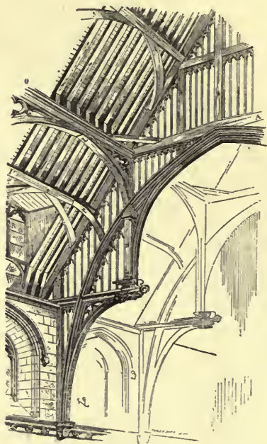
FIG. 166 A. London, England: Westminster Hall. Part of the roof seen from within. About 1398 A.D. O , principal horizontal piece which bears upon the vertical posts D , and which carries the rafters about half-way between the wall-plate and the ridge. The vertical posts D rest upon the hammer-beams, the ends of which are carved into figures of angels. A , collar-beam, which is a horizontal tie. I, I' , secondary horizontal pieces or purlines. L, N, P , diagonal braces. R , dormer window.
