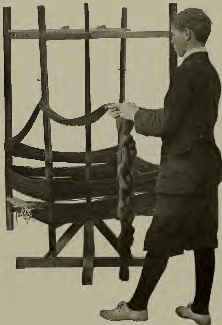
Fig. 15—Removing the Warp from the Reel
