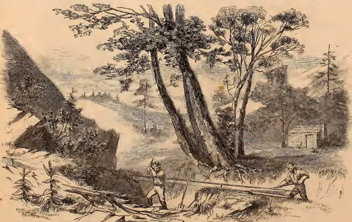
MINERS WASHING THEIR GOLD DIRT THROUGH THE "LONG TOM"—A SCENE NEAR SACRAMENTO, CALIFORNIA.
