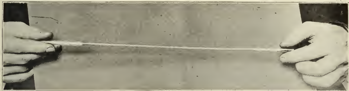
Fig. 5.—Method of drawing out pipets.
