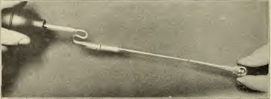
Fig. 12.—Filling bulbs with vaccine with a 1 c.c. pipet.
