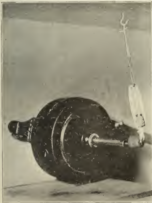
Fig. 9.—Shaker for breaking up clumps of tubercle bacteria.
