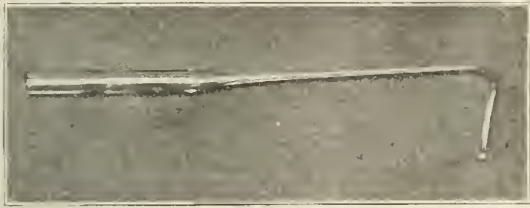
Fig. 8.—Glass rod for spreading the incubated mixture on the slide.
