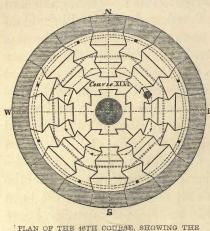
PLAN OF THE 46TH COURSE, SHOWING THE METHOD OF DOVETAILING.
