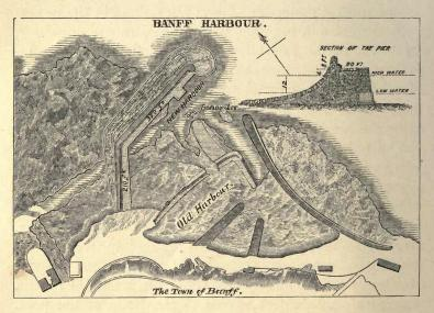
This harbour occupies the triangular space at the north-eastern extremity of the projecting point of land, at the opposite side of which, fronting the north-west, is the little town and harbour of Macduff. In 1816 Mr. Telford furnished a plan of a new pier and breakwater, covering the old entrance, which presented an opening to the N.N.E., with a basin occupying the
