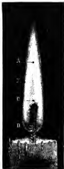
FIG. 36.—In the candle flame the portion C contains the vapours and products of decomposition; in the bright zone A the combustion has commenced, and particles of carbon are emitted; and in the pale zone B the combustion is completed.
