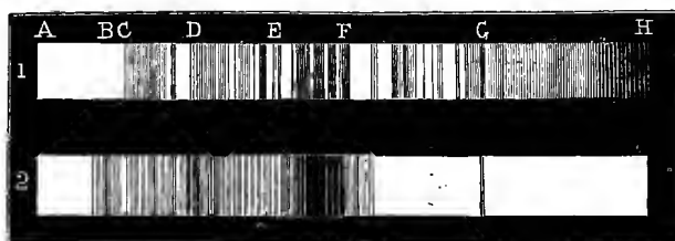
FIG. 74.—Absorption spectra of nitrogen dioxide and iodine.
