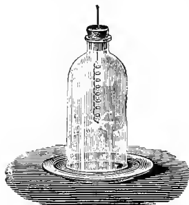
FIG. 30.—Mode of burning a steel spring in oxygen.
