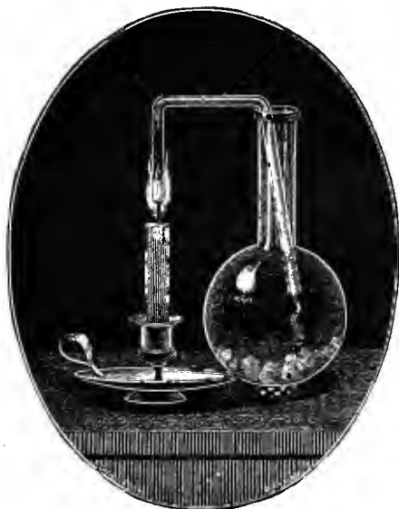
FIG. 35.—Faraday's experiment for investigating the different parts of a candle flame.
