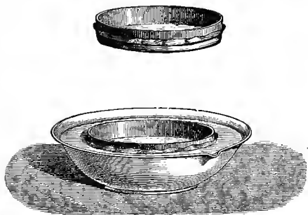
FIG. 15.—Dialyser. Apparatus for the separation of substances which pass through a membrane from those which do not. Description in text.
