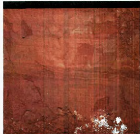
Figure 7. Thin strata near Test Pit 3 in chamber 5. Note the darker and lighter sections. The darker lenses probably contain greater amounts of organic debris. The white material at the base of the profile are calcite crystals that appear to represent bedrock. The top of the profile is present ground surface. This section is about 80cm deep.
