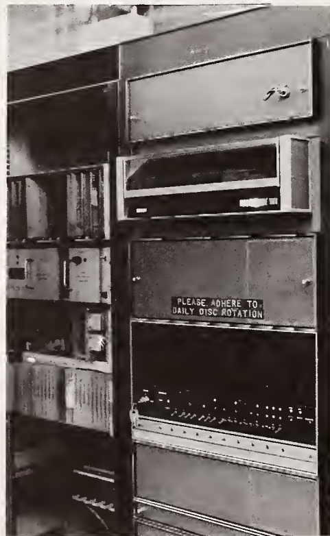
FIGURE 5-11: ANN ARBOR COMPUTER SYSTEM. On right, top to bottom: disc unit, computer and communications multiplexer
