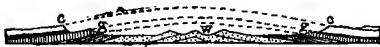
FIG. 84.—Section across the Weald from North to South. cc Chalk, g Greensand escarpments, w Wealden sandstones
