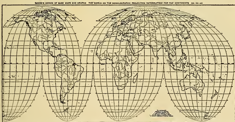
Miniature of Map No. 101 Hc. The homolographic projection, interrupted to present the continents The entire earth's surface is shown without distortion of area
