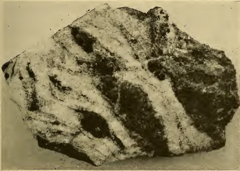
FIG. 1.—Inclusions of clinopyroxene skarn in aplitic gneiss. E. of Benson Pond, Washington, Massachusetts. Eight-ninths natural size.
