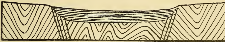
FIG. 2.—Diagram representing a depression developed by faulting which was continuous during the period of sedimentation.
