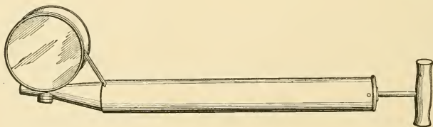
FIG. 15. Cologne Vaporizer used to determine the rate of circulation of air in the New York Subway.
