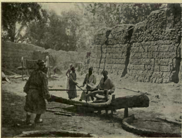
How wheels for the arba are made.
