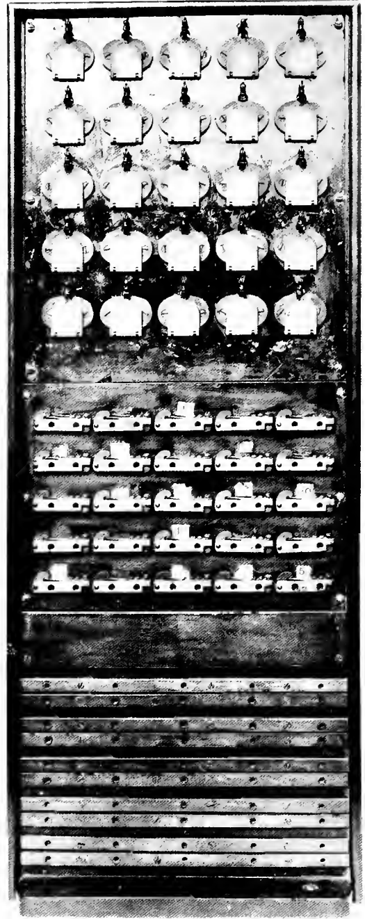
The Universal Switchboard Manufactured by the Western Electric Co. under Charles E. Scribner's Patent, and from which the Standard Switchboard Developed
