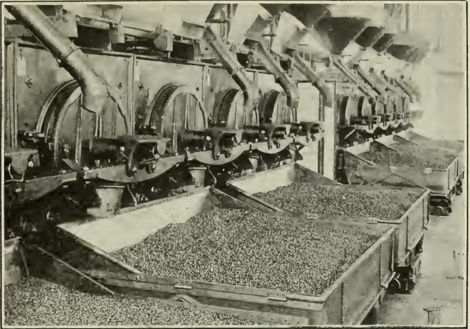
FIG. 1.—PEANUTS FOR MAKING PEANUT BUTTER ARE ROASTED IN REVOLVING DRUMS, THEN DUMPED INTO LARGE TRAYS AND COOLED BY A BLAST OF COLD AIR.
