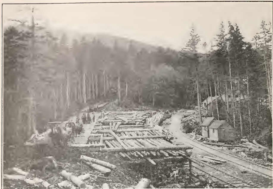
SKIDWAY WITH FOUR-HORSE TEAMS UNLOADING, SCALER SCALING LOGS, AND THREE LOADED CARS ON TRACK; NEW CAMP ON RIGHT. LINCOLN, N. H.
