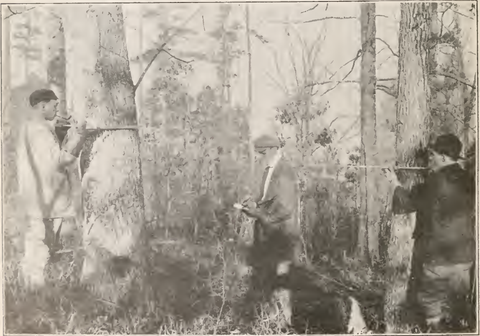
CALIPERING TREES IN A MIXED HARDWOOD STAND, COLLEGE FOREST, UNIVERSITY OF GEORGIA
