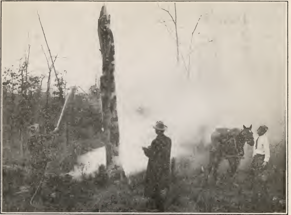
TESTING CHEMICAL ENGINE ON A BURNING TREE SNAG, THE IN- VENTOR, MR. ADAMS, IN FORE- GROUND
