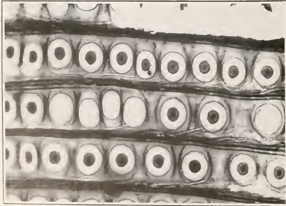
FIG. 7. RADIAL SECTION MAGNIFIED 800 TIMES SHOWING BORDERED PITS. THE TORUS IS VISIBLE IN MANY OF THESE, APPEARING AS A BLACK OVAL DISK IN CENTER OF PIT
