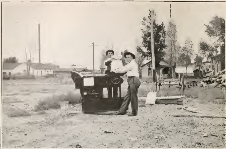
FOREST OFFICERS OPERATING A FANNING MILL, THROUGH WHICH SEED IS RUN FOR ITS FINAL CLEANING. ALL DUST, BROKEN WINGS, AND LIGHT SEED ARE BLOWN OUT FROM GOOD SEED
