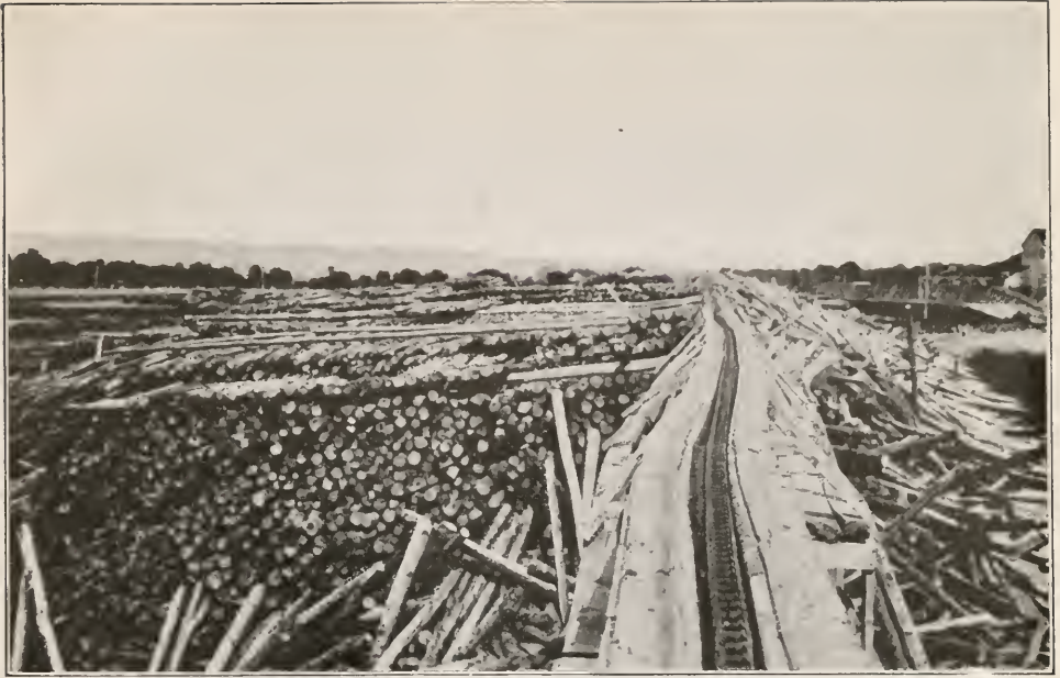
No. 7. THE SMALL TREES AND TOP LOGS USED IN THE ROUND FOR MINE TIMBERS ARE LIFTED FROM THE POND TO THE MILL YARD BY THE CHAIN CONVEYOR.
