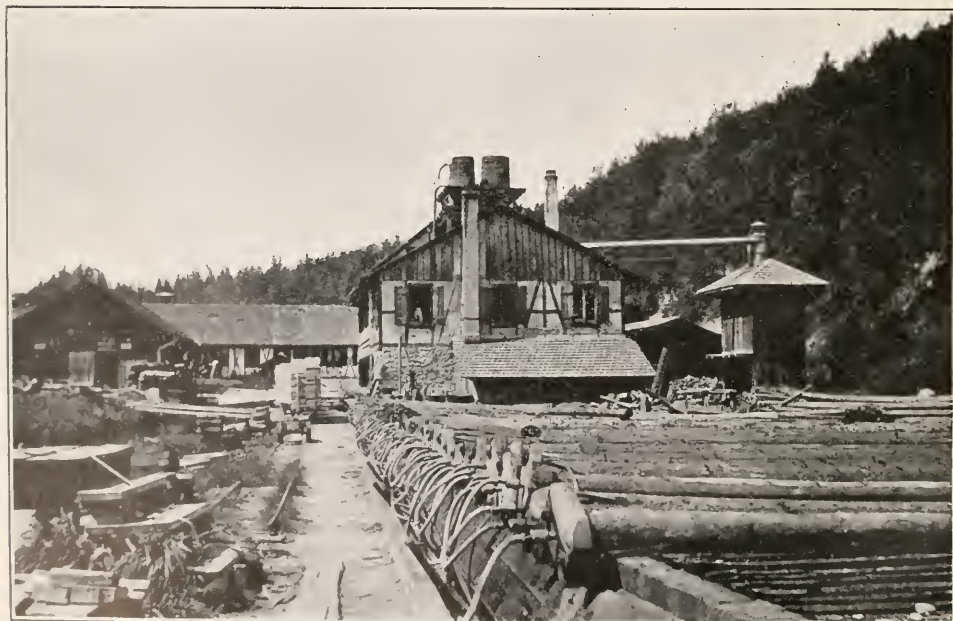
THE SAWMILL AND TREATING PLANT. IN THE RIGHT FOREGROUND ARE SPRUCE POLES BEING TREATED BY THE BOUCHERIE PROCESS; THE COPPER SULPHATE COMES FROM THE TANKS ON THE BUILDING IN THE BACKGROUND. THIS BUILDING CONTAINS THE TURNING LATHES, EXCELSIOR MACHINE, AND CORDWOOD SPLITTER. THE LOW BUILDING ON THE LEFT IS THE SAWMILL. IN THE LEFT FOREGROUND MAY BE SEEN THE CANAL BY WHICH THE WATER IS DIVERTED FROM THE RIVER TO GIVE THE POWER
