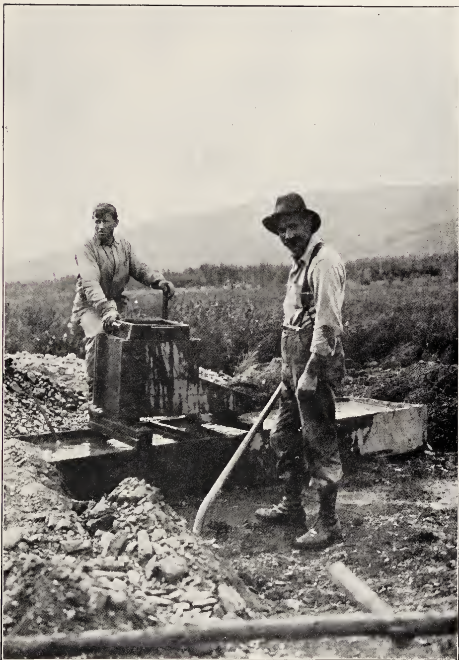
To-day most of the Klondike gold is recovered by machinery in large-scale workings, but now and then one sees a miner washing the gravel by hand in a contrivance like this.
