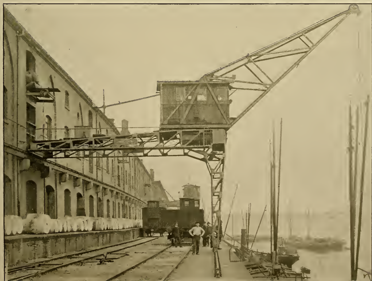
FIG. 8.—ELECTRICALLY-DRIVEN "ANGLE PORTAL" CRANE AT MANNHEIM, GERMANY. CAPACITY, 1\frac{1}{4} TONS; 29 FT. 6 IN. RADIUS. BUILT BY THE NAGEL & KAEMP IRONWORKS CO.
