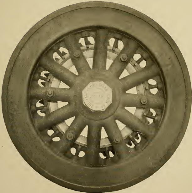
FIG. 5.—COMPOSITE WHEEL MADE BY THE LANCASHIRE STEAM MOTOR COMPANY, LTD., LEYLAND
