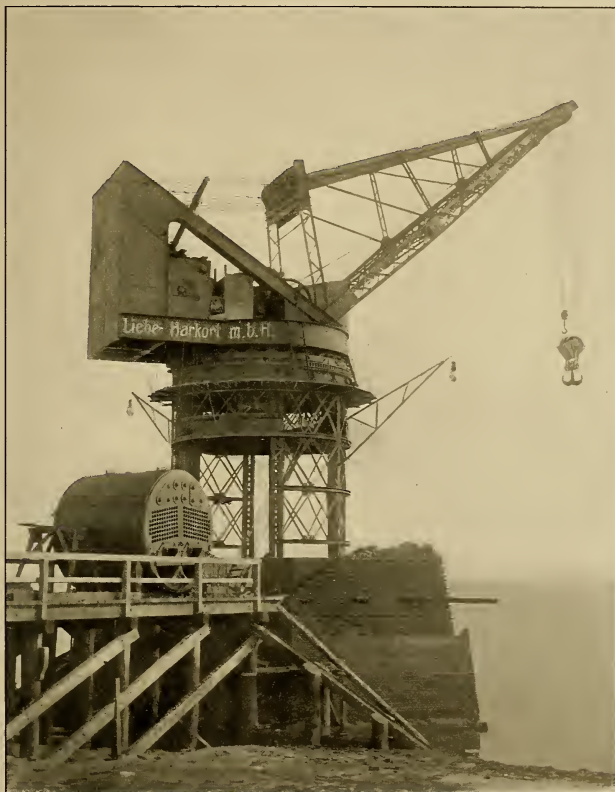
FIG. 17.—A 75-TON ELECTRIC REVOLVING CRANE BUILT BY THE DUESSELDORFER KRAHNBAUGESELLSCHAFT LIEBHERR-HARKORT, M. B. H.
