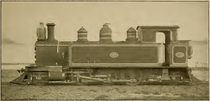
FIG. 10.—GOODS TANK LOCOMOTIVE FOR HEAVY GRADIENTS, CLASS "wa," BUILT IN THE NEW ZEALAND RAILWAY WORKSHOPS. CYLINDERS, 14 IN.; STROKE, 20 IN.; DIAMETER OF DRIVING WHEELS, 3 FT. 3\frac{3}{4} IN.; TRACTIVE POWER, 11,833 LBS.; TOTAL WEIGHT IN WORKING TRIM, 37\frac{1}{4} TONS
