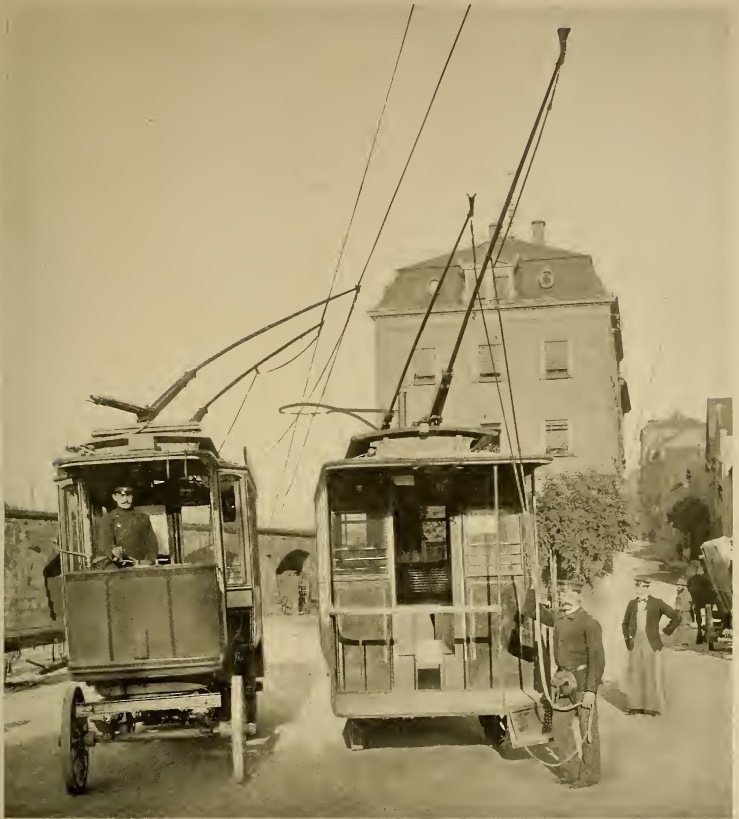
ONE OF THE OMNIBUSES HAS ITS TROLLEY POLES PULLED DOWN, SO AS TO LET THE OTHER VEHICLE PASS
