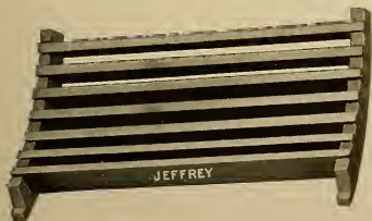
FIG. 3.—A SECTION OF THE SCREEN FRAME OF THE JEFFREY PULVERISER
