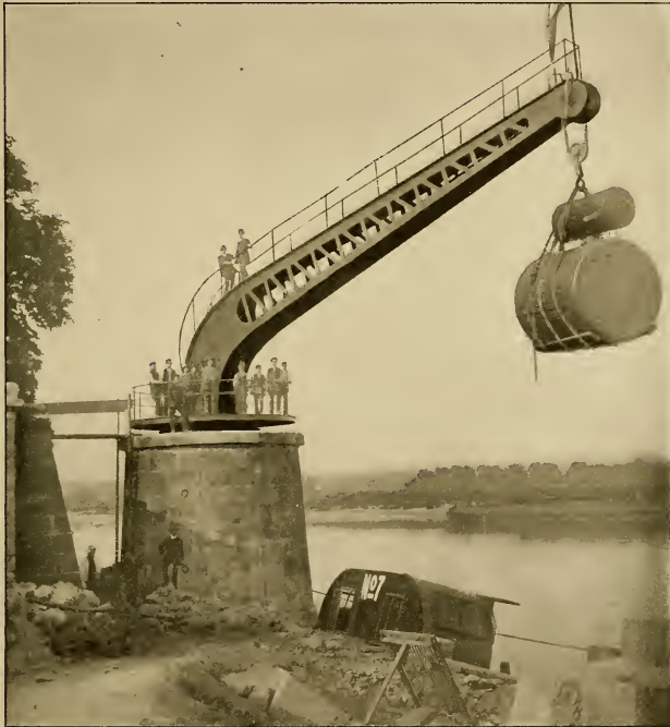
FIG. 13.—A 25-TON ELECTRIC REVOLVING WHARF CRANE, 44 FEET RADIUS, BUILT BY THE NAGEL & KAEMP IRONWORKS CO., HAMBURG, GERMANY
