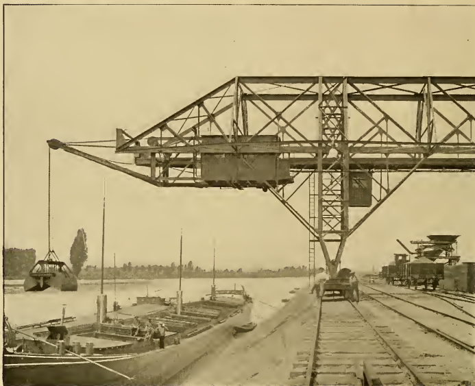
FIG. 5.—ELECTRICALLY OPERATED JIB AT THE END OF A COAL-HANDLING CRANE, INSTALLED BY THE ELECTRICAL ENGINEERING CO., LTD., LONDON
