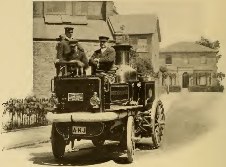
A SELF-PROPELLED STEAM FIRE ENGINE, BUILT BY MESSRS. MERRYWEATHER & SONS, LTD., LONDON
