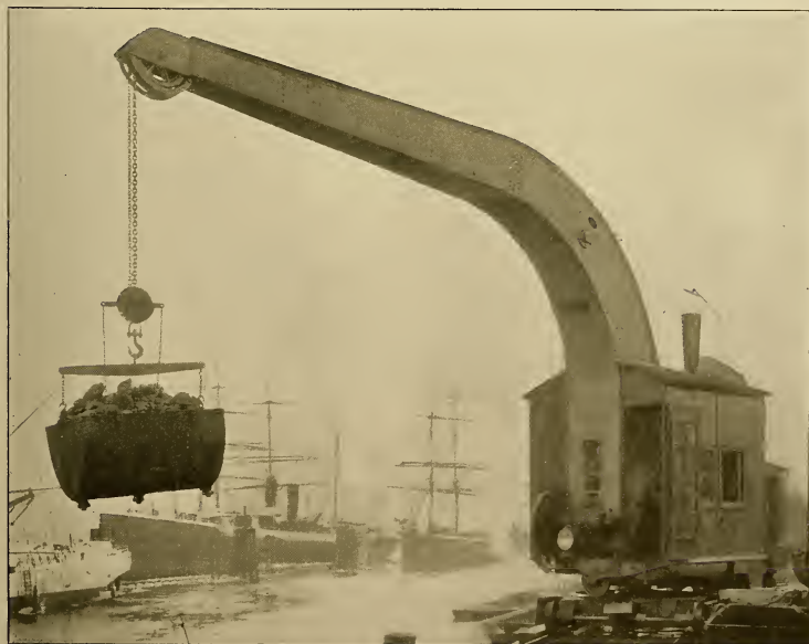
FIG. 11.—A 2½-TON STEAM CRANE, ON THE HAMBURG DOCKS. BUILT BY MESSRS. MOHR & FEDERHAFF, MANNHEIM, GERMANY
