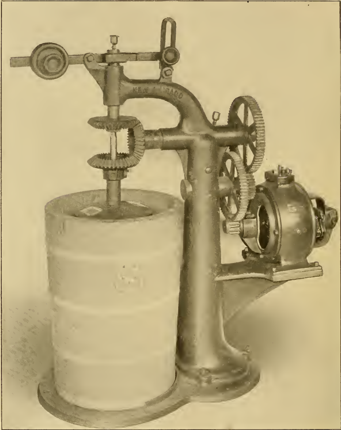
FIG. 11.—ICE-CREAM FREEZER DRIVEN BY A WESTERN ELECTRIC COMPANY (CHICAGO) MOTOR
