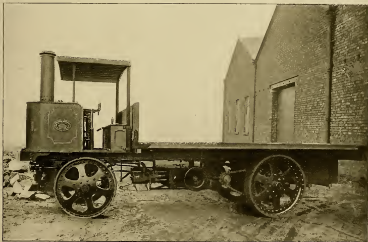
FIG. 7.—THE WHEELS HERE HAVE SPOKES MADE OF STEEL PLATES CUT SO THAT ALL THE SPOKES ON EACH SIDE ARE IN ONE PIECE. MADE BY THE LANCASHIRE STEAM MOTOR CO., LTD.
