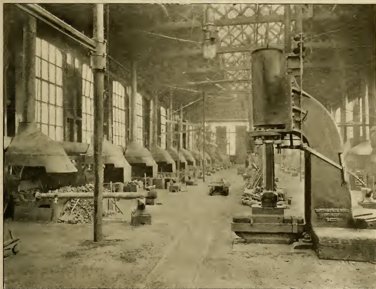
THE SMITH'S SHOP AT HARLAND & WOLFF'S YARD, BELFAST. THE STEAM HAMMERS HERE SHOWN ARE FROM THE WORKS OF MESSRS. DAVIS & PRIMROSE, LTD., LEITH
