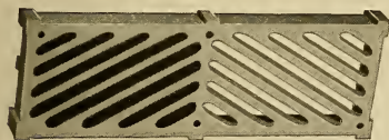
FIG. 2.—A SECTION OF THE SCREEN FRAME OF THE JEFFREY PULVERISER FOR HEAVY WORK
