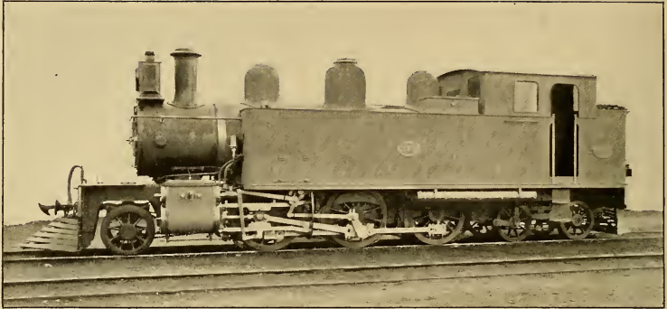
FIG. 13.—SUBURBAN TANK LOCOMOTIVE, CLASS “wf,” BUILT IN THE NEW ZEALAND GOVERNMENT RAILWAY WORKSHOPS. CYLINDERS, 14 IN.; STROKE, 22 IN.; DIAMETER OF DRIVING WHEELS, 3 FT. 9 IN.; TRACTIVE POWER (AT 75 PER CENT. BOILER PRESSURE), 14,370 LBS.; BOILER PRESSURE, 200 LBS.; TOTAL WEIGHT IN WORKING TRIM, 4\frac{3}{4} TONS; GAUGE, 3 FT. 6 IN.
