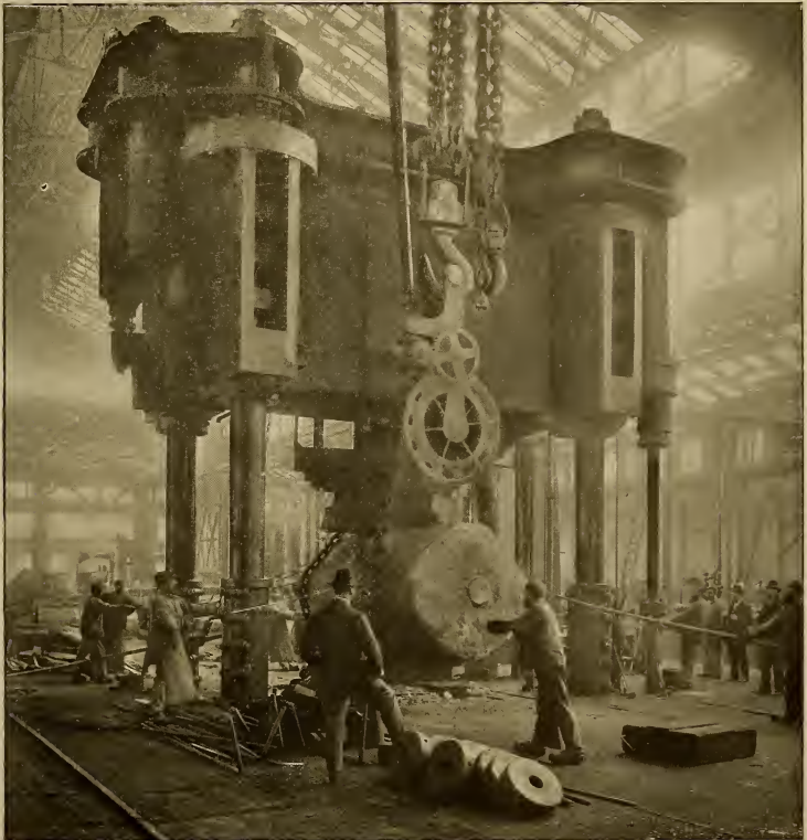
UNDER THE 5000-TON HYDRAULIC FORGING PRESS AT THE ESSEN WORKS
