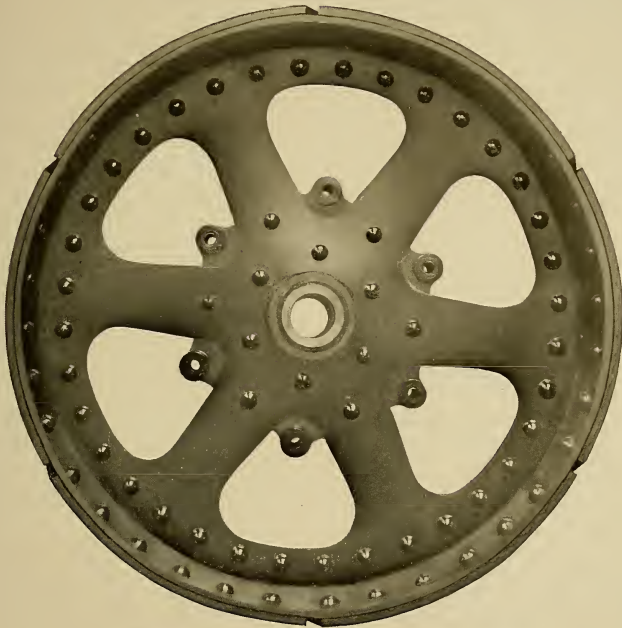
FIG. 11.—A DOUBLE PLATE WHEEL MADE BY THE LANCASHIRE STEAM MOTOR CO., LTD.
