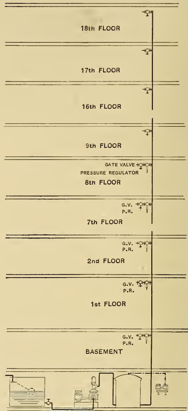
FIG. 6.—PRESSURE TANKS IN THE BASEMENT
