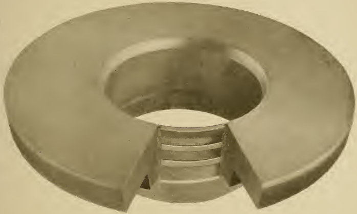
FIG. 3.—AN EXAMPLE OF COLD-FLOWED STEEL JOINT. A SECTION OF THIS FLANGE HAS BEEN CUT AWAY TO SHOW HOW THE METAL HAS FLOWN INTO THE RECESSES
