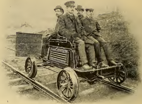
AN AUTOMOBILE FOR INSPECTION SERVICE ON STEAM RAILROADS. BUILT BY THE OLDS MOTOR WORKS, DETROIT, MICH.
