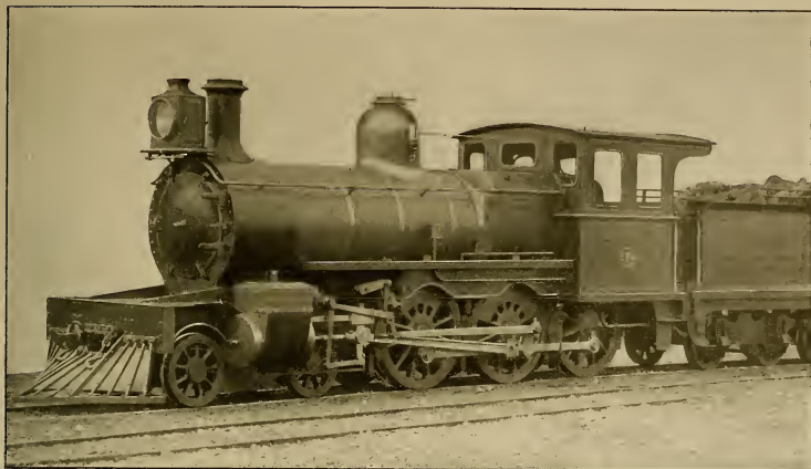
FIG. 6.—EXPRESS PASSENGER LOCOMOTIVE, CLASS "U," BUILT IN THE NEW ZEALAND RAILWAY WORKSHOPS. CYLINDERS, 16 IN.; STROKE, 20 IN.; DIAMETER OF DRIVING WHEELS, 4 FT. 6 IN.; DIAMETER OF BOGIE WHEELS, 2 FT. 6 IN.; TRACTIVE POWER, 12,400 LBS.; TOTAL WEIGHT IN WORKING TRIM, 61 TONS
