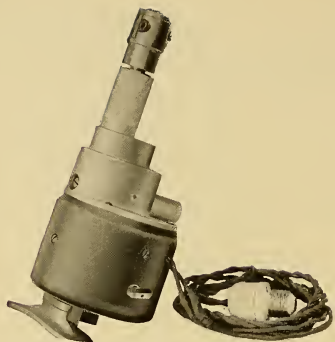
FIG. 28.—AN ELECTRICALLY DRIVEN BREAST DRILL
