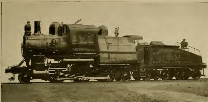
THE FIRST ANTHRACITE COAL-BURNING LOCOMOTIVE IN THE AMERICAN SOUTHERN STATES FOR BURNING VIRGINIA ANTHRACITE. BUILT BY THE RICHMOND, VA., WORKS OF THE AMERICAN LOCOMOTIVE COMPANY
