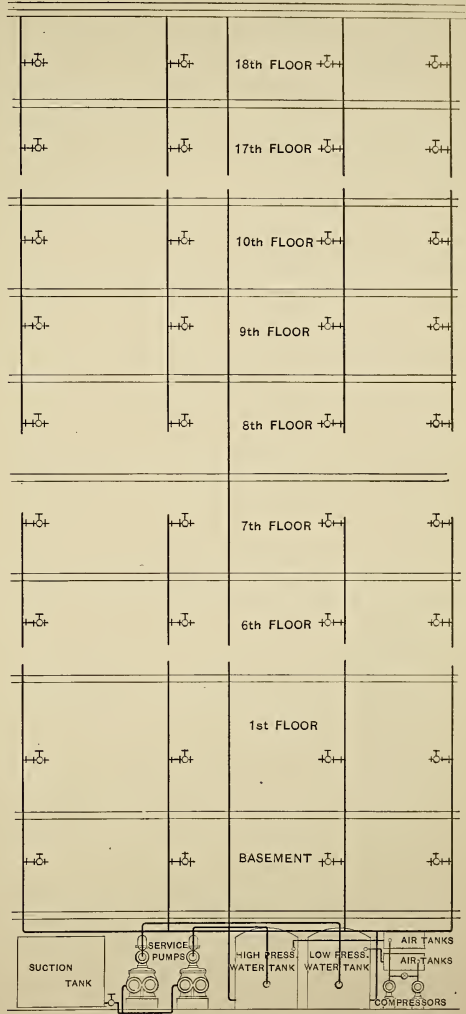
FIG. 7.—SEPARATE PUMPS AND PRESSURE TANKS FOR THE UPPER, INTERMEDIATE AND LOWEST FLOORS
