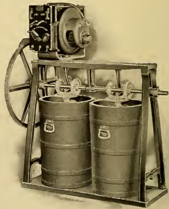
FIG. 8.—AN ELECTRICALLY DRIVEN DOUBLE ICE-CREAM FREEZER, MADE BY F. E. WHITNEY, BOSTON, MASS. THE MOTOR IS OF GENERAL ELECTRIC MAKE
