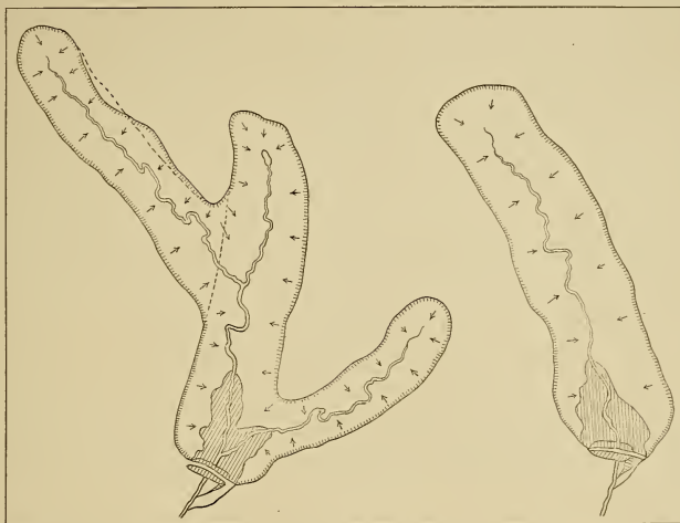
FIGS. 7 AND 8.—SURFACE WATER IMPOUNDED BY A DAM IN THE CASE OF A MAIN AND TWO SIDE VALLEYS, AND ALSO IN THE CASE OF A SINGLE VALLEY
