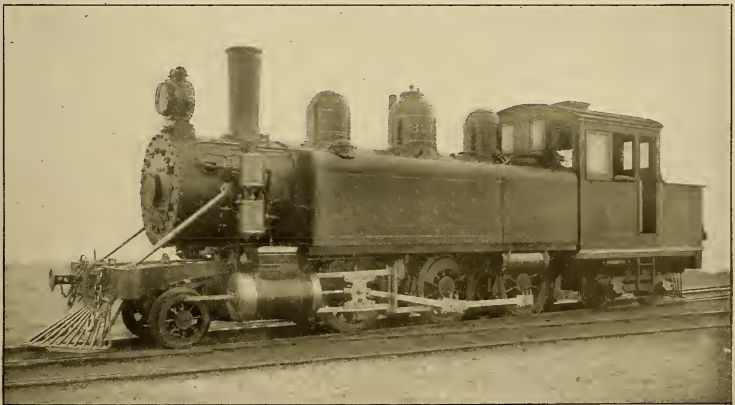
FIG. 11.—GOODS TANK LOCOMOTIVE FOR HEAVY GRADIENTS, CLASS "wd," BUILT AT THE BALDWIN LOCOMOTIVE WORKS, PHILADELPHIA, U. S. A. CYLINDERS, 14 IN.; STROKE, 20 IN.; DIAMETER OF DRIVING WHEELS, 3 FT. 3\frac{3}{4} IN.; TRACTIVE POWER, 14,790 LBS.; TOTAL WEIGHT IN WORKING TRIM, 43\frac{3}{4} TONS
