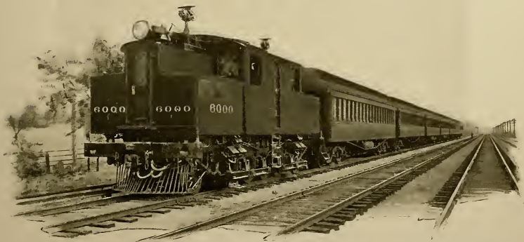
ONE OF THE 95-TON ELECTRIC LOCOMOTIVES BEING BUILT TO SUPPLANT STEAM LOCOMOTIVES ON TWO DIVISIONS OF THE NEW YORK CENTRAL RAILROAD
