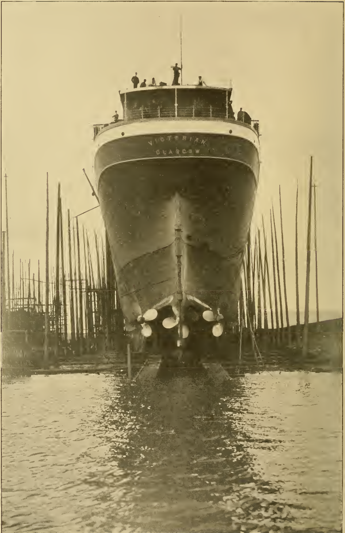
A STERN VIEW OF THE "VICTORIAN" BEFORE LAUNCHING. THE CENTRAL PROPELLER IS DRIVEN BY A HIGH-PRESSURE TURBINE; THE TWO OTHERS BY LOW-PRESSURE TURBINES
