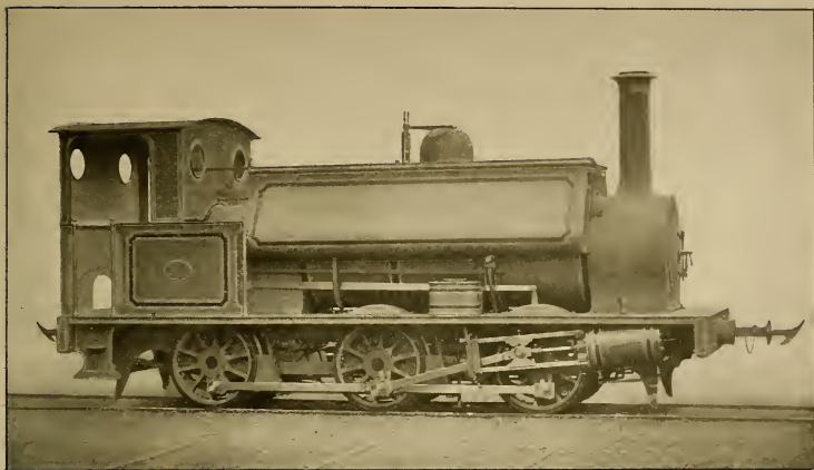
FIG. 4.—NEW ZEALAND ENGINE, CLASS "F." THE MOST NUMEROUS IN THE COLONY. CYLINDERS, 10\frac{1}{2} \times 18 IN.; WHEELS, 3 FT.
