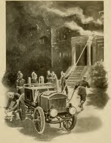
AN ELECTRICALLY PROPELLED AND MOTOR-DRIVEN FIRE-PUMP, ALSO OF MERRYWEATHER MAKE
