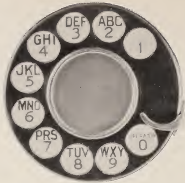
FIG. 33.— The dial—panel-type system
