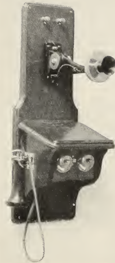
FIG. 13.—A common-battery telephone
