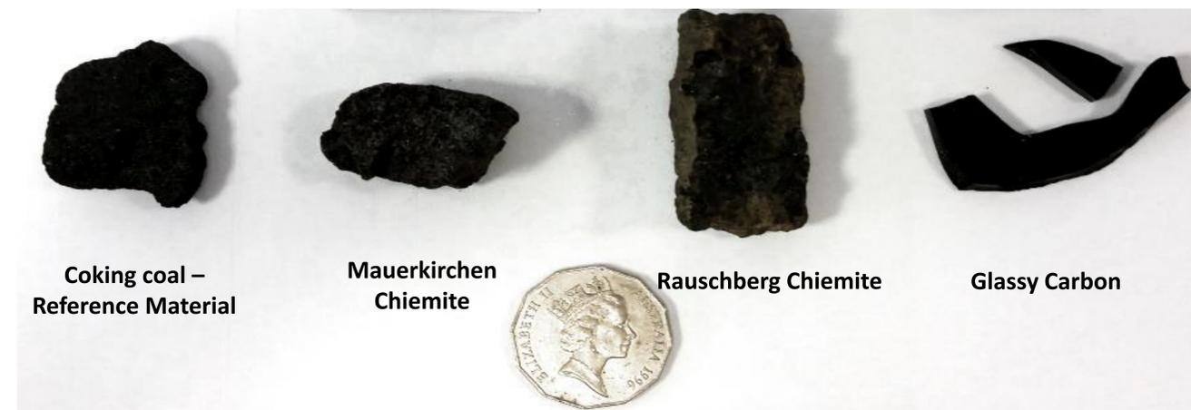
Figure 1: Samples analysed: Coking Coal reference material, Mauerkirchen Chiemite, Rauschberg Chiemite, Glassy Carbon.
