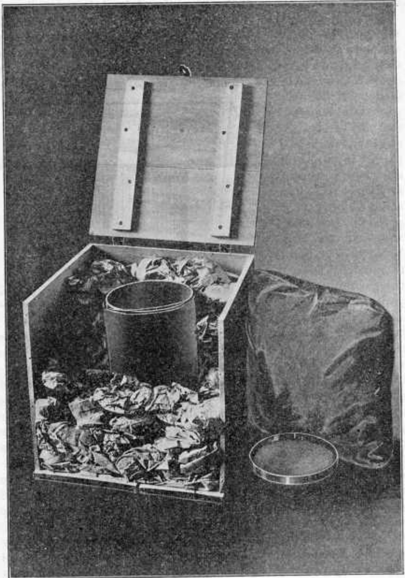
FIG. 4.—Homemade fireless cooker with part of outside container removed to show packing of crumpled paper and the cooking vessel, with its container.
