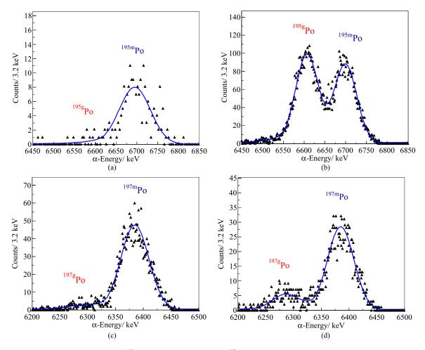
FIG. 4. The  $\alpha$ -decay energy spectra for <sup>195</sup>Po, panels (a) and (b), and <sup>197</sup>Po, panels (c) and (d), measured with the two silicon detectors surrounding the implantation point in DSS2.0. The spectra were recorded at different RILIS wave numbers: Panels (a) and (c) were taken at 11853.75 and 11853.95 cm<sup>-1</sup> respectively, while panels (b) and (d) were taken at 11853.83 cm<sup>-1</sup>.
