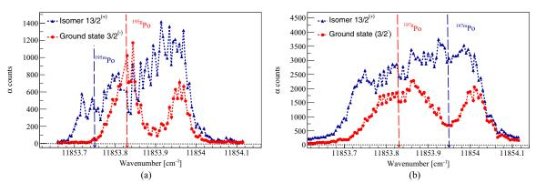
FIG. 3. The hyperfine structure of the 843-nm atomic transition for the  $3/2^-$  and  $13/2^+$  nuclear states in (a) <sup>195</sup>Po and (b) <sup>197</sup>Po [26,32]. The dashed lines indicate the wave numbers used for the mass measurements. Note that the two hyperfine spectra were recorded in a different experiment, and hence the laser resolution achieved in the present work is different.
