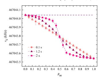
FIG. 7. Center frequency  $v_c$  resulting from a fit of a mixed resonance with a single-resonance curve, as a function of the isomeric state ratio  $R_m$ . It was obtained from simulated data of <sup>195</sup>Po for different excitation times. The purple dashed straight line represents the pure cyclotron frequency of the ground state where the ratio of ground-to-isomeric state is 1:0.
