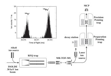
FIG. 2. Schematic view of the ISOLTRAP setup with the  $\alpha$ -decay station. Inset: time-of-flight spectrum of mass A = 195. Full separation of <sup>195</sup>Po<sup>+</sup> from <sup>195</sup>Tl<sup>+</sup> isotopes was achieved after 1000 revolutions in the MR-ToF MS.
