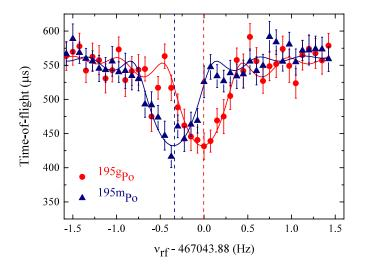
FIG. 5. ToF-ICR resonances of  $^{195(g,m)}$ Po with 2 s excitation time in red circles (ground state) and blue triangles (isomeric state). The red (blue) dashed line represents the center frequency of the ground (excited) state. Quasipure samples of either state were measured thanks to selective enhancement from RILIS and different half-lives (see text for details). The solid lines represent the fit of the theoretical line shape [41] to the experimental data.
