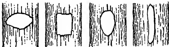
Four incisions in trees, the one at the left being the most damaging and slowest to heal; the one at the right least damaging and quickest to heal
