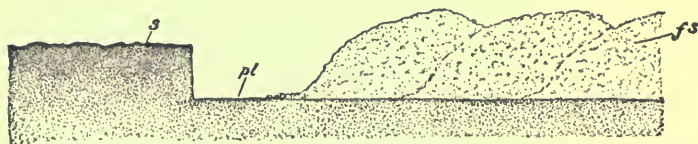
FIG. 11.—Land before and after plowing. The compactness of the soil is indicated by the density of dotting. Before plowing there is a compact surface crust ( s ), below which the soil becomes less and less compact as we go deeper. After plowing we find the soil ( fs , furrow-slice) converted into a loose mass of crums (flocules), with increase of bulk. Compacted plow-sole at pl
