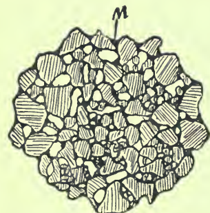
FIG. 12.—A soil-crumb, magnified to show the particles of which it is composed. The particles are held together by the water-menisci, just as are the hairs of a brush when wetted. The white spaces between the particles represent air.
